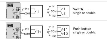
Local control wires can be extended up to 10 m (separate from the 230 V).
