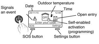
Before any operation, you must "activate" the display by pressing the button.
