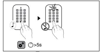
Press and hold the 🕑 button for 5 seconds until the green LED comes on.
