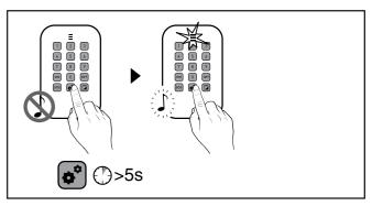
To enable the beeps again, press the solution for 5 seconds.
