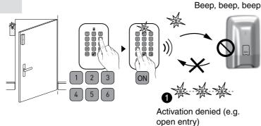
Enter your access code a second time then press **ON** within 5 seconds after first pressing the button. The LED changes from red to green to confirm the action. The alarm control unit emits a BEEP.
