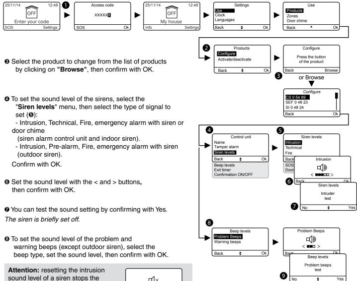
sound level of a siren stops the siren form sounding in the event of: - intrusion,
