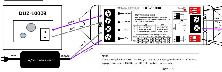
Set signal type to passive dimmer, and dimming curves with DIP switches.
