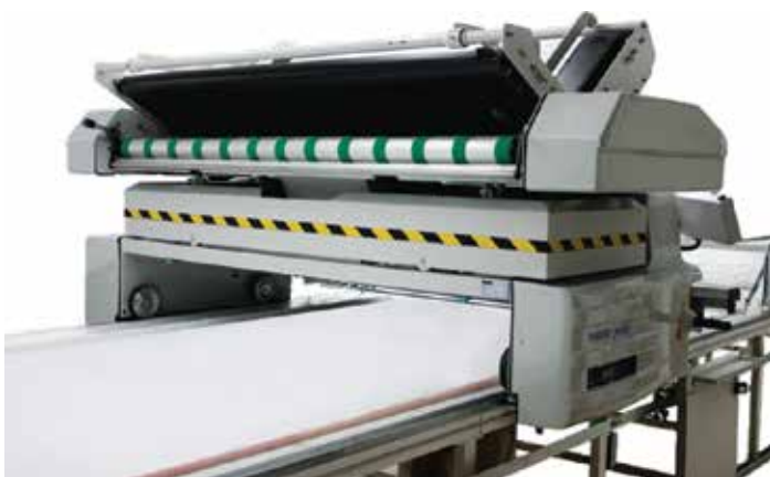
Cradle Feed System Provides Tension-Free Spreading
