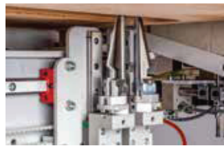
Precision-enhanced corner knife system with stepper motor
