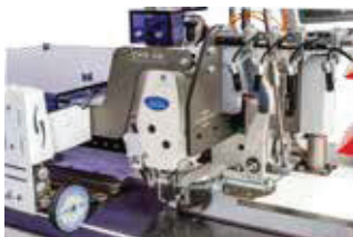
Precision-enhanced interlining unit with stepper motor
