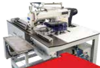
Easy screen adjustment due to one-on-one synchronous motors
