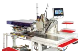
Precision-enhanced corner knife system with stepper motor
