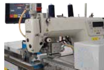
Standard dimensions in sewing lengths with vacuum unit fixing fabrics
