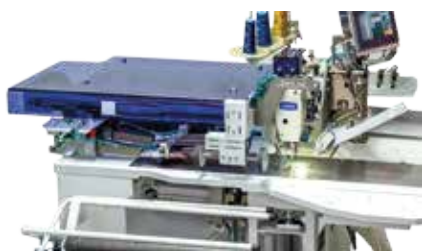
Precision-enhanced interlining unit with step-per motor inclined stitching range from 0.1 to 8 mm
