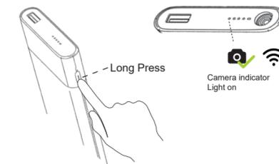
Long press 1.5 sec, the camera indicator light will be solid white. Waiting for 40 seconds, the camera indicator light will blink, and the camera system will launch signal. In 20 sec, the camera light will be off.
