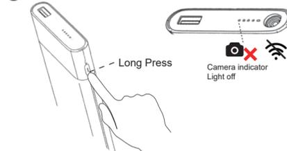
Long press 3 sec, the camera indicator light will turn off. Waiting for 10 seconds, the camera system will be closed.
