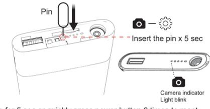
Pin for 5 sec or quickly press power button 6 times to reset. The camera light will blink, and the camera will be resetted. You can only Wi-Fi direct view within a certain range.
