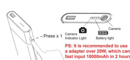
Press power button once, the light is on, you can check the battery level and whether the camera indicator light is working
