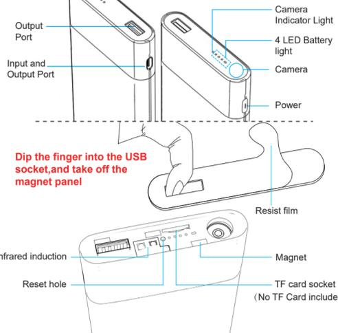
Dip the finger into the USB socket, and take off the magnet panel
