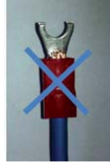
Terminal has been cut.
