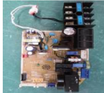
Connection of terminal block and Main PBA
