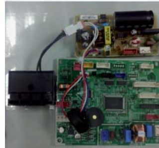
Connection of terminal block and Main PBA
