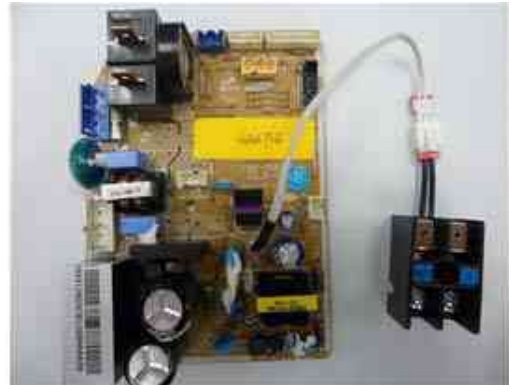
Connection of terminal block and Main PBA
