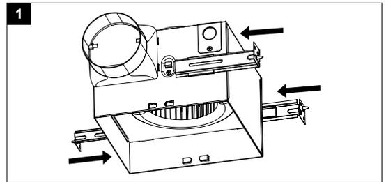
2. Mount the fan body to joist using the suspension brackets and long wood screws.
