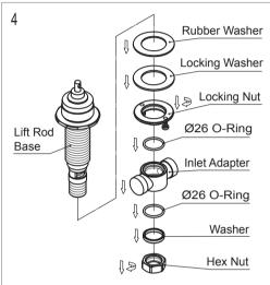
Take off the following from the lift rod base accordingly: the hex nut, washer, Ø26 O-Ring, inlet adapter, locking nut, locking washer and rubber washer.
