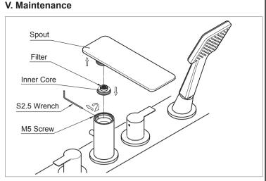
After a period of usage, if the volume lessens, it might be due to debris from bad quality water blocking the inner core. Loosen the M5 screw and take out the spout and then the inner core. Clean its filter with clean water. Then install it back.
