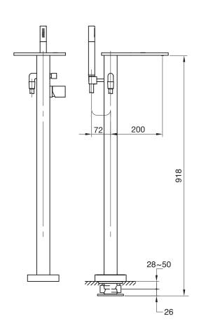
Includes rough-in 6 GPM (22.7 L/min.)
