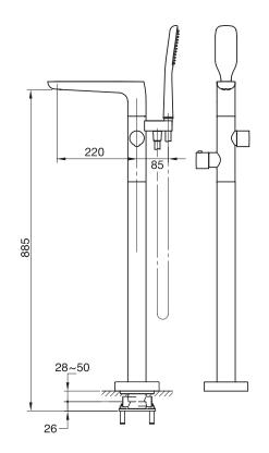
Includes rough-in Thermostatic control 5 GPM (18.9 L/min.)
