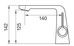
Lead free brass Includes push drain 3/8" flexible supply hoses 1.75 GPM (6.6 L/min.)
