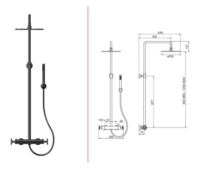
Exposed thermostatic mixer with 2-way diverter Includes 9 3/4" rain head, hand shower and hose Hand shower on separate hook Rainhead: 2.2 GPM (8.3 L/min.)
