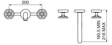
Includes rough-in Includes push drain 1.5 GPM (5.7 L/min.)
