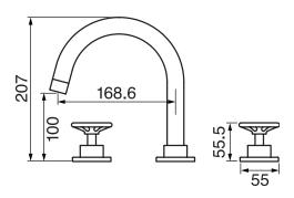
Includes push drain 1.5 GPM (5.7 L/min.)
