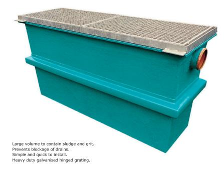
For ease of access and to empty the VW silt trap the grating is hinged and held open with an integral stay. Sludge can then be removed manually or by tanker.
