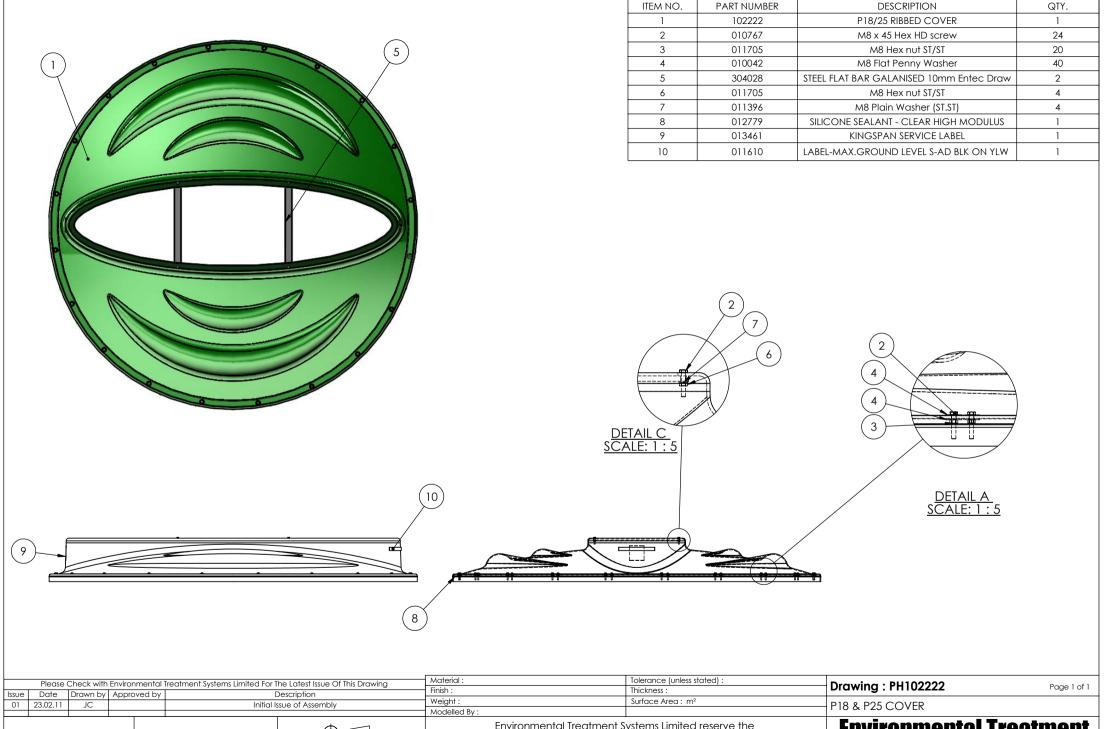
Scale: Do Not Scale Z:\engineering\Drawing Data\04 - Sub Assembly\100 - 000 Laminated Components\1022\PH102222
