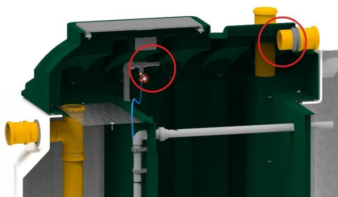
Figure 5: Airline connections inside and outside the tank for CAP 6 and CAP 12 models
