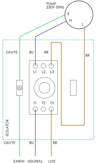
SEWAGE PUMP GRUNDFOS UNILIFT AP50B.50.08.A1.V 230V 50Hz 5.37 Amp
