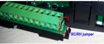
• If the HVAC system contains separated heating and cooling transformers, please cut out the RH/RC jumper and then connect the RC and RH inputs individually.
