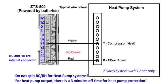
Figure 12. Heat pump 2-wires HVAC system wiring
