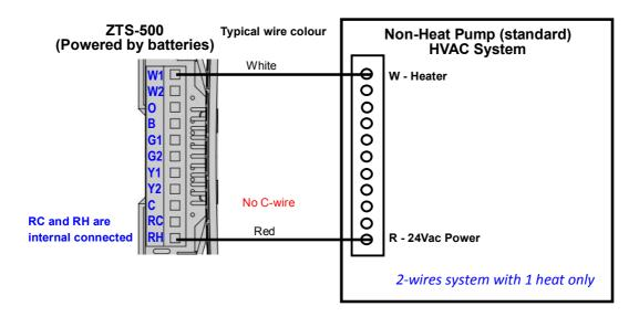
Figure 9. Non-heat pump (Standard Gas or Electric) 2-wires HVAC system wiring
