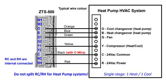
Figure 11. Heat pump HVAC system wiring
