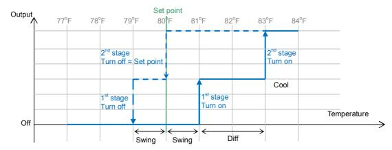
**AUTO mode:** Thermostat controls the temperature according to the following diagram.
