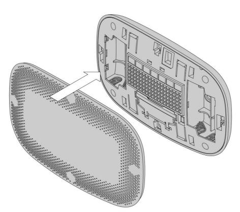
Figure 5. Install the front housing
