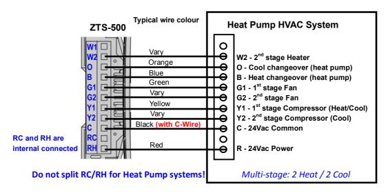
Figure 10. Heat pump HVAC system wiring
