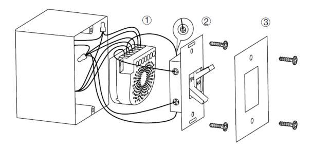
**Note:** 1. The gang box should be sized  $3\times2\times2.75$  inch /  $75\times50\times70$  mm or larger, minimum volume 14 in / 230mm.
