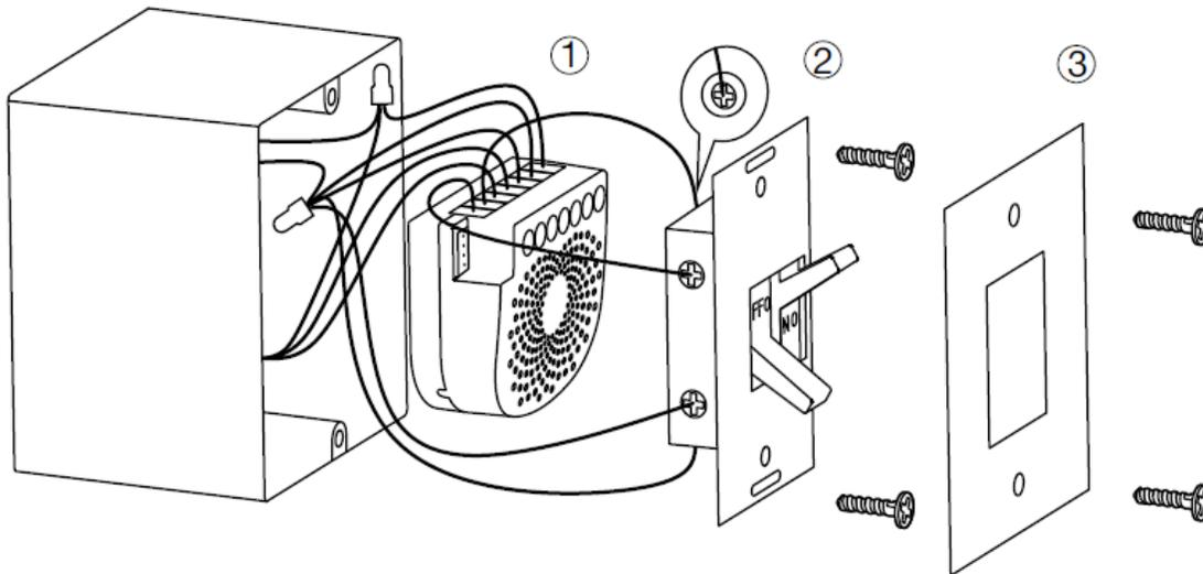
**Note:** 1. The gang box should be sized 3x2x2.75 inch / 75x50x70 mm or larger, minimum volume 14 in / 230mm.
