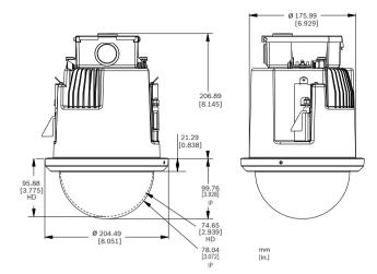
Fig. 2: AUTODOME 7000 series In-ceiling
