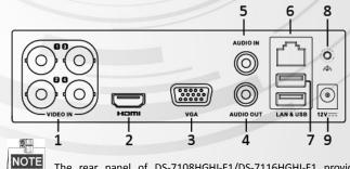
The rear panel of DS-7108HGHI-F1/DS-7116HGHI-F1 provides
