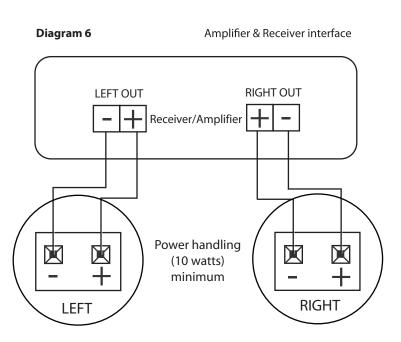
Note: Speaker terminals have corresponding (+) and (-) terminals. It is important to connect both speakers in phase. Out of phase will result in thin sound and weak bass.
