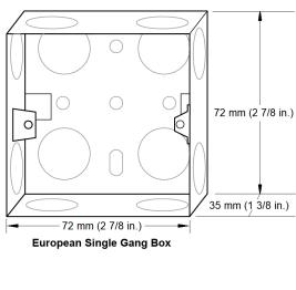
The European Single Gang Box has a minimum depth of 35 mm (1 3/8 in.). Use the box with only two mounting tabs. Supplied separately.
