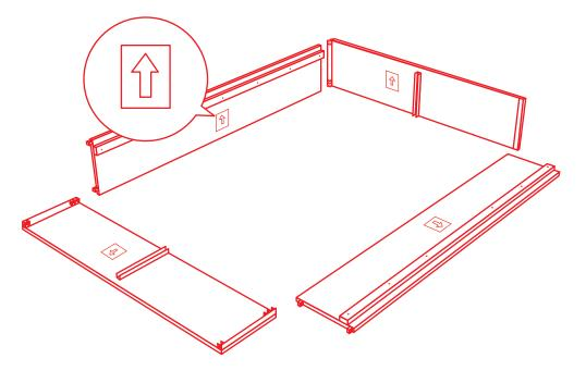
Fasten the interlocked joints by inserting one pin at the top of the joint and a second pin at the bottom of the joint.
