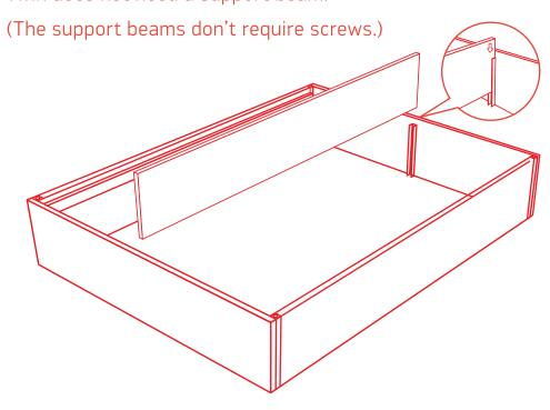
Place the support rod into the 2 holes that are located in the center of the 2 side support beams. (No screws needed)
