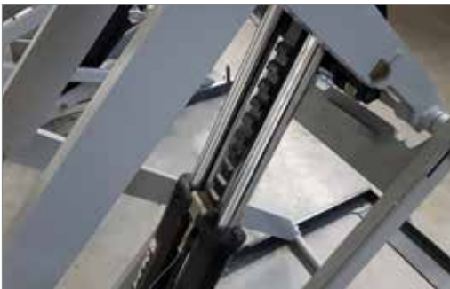
MECHANICAL SAFETY LOCK SICURA MECCANICA
