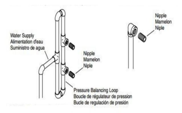
2) Finished Tile wall installation holes (for wall mounted shower systems)
