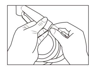
4. Wrap the angle valve with PTFE tape to prevent leakage.
