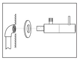
6. Make sure that the rubber pad is firmly fixed inside the hose and then connect the hose to the angle valve.
