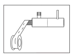
5. Connect the angle valve to the water supply pipe.
