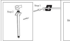
Step 1. Wrap the teflon tape on the thread Step 2. Clockwise rotation of the ceiling arm to the pipe
