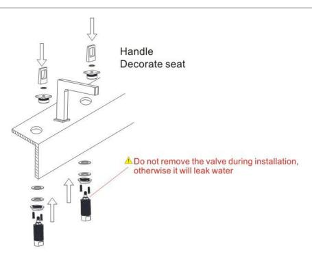
Remove the Decorate Seats and put them on the basin holes. Connect the Control Water Bodies with Decorate Seats from the underside of the basin holes, and tighten them. Finally install the Handles and tighten them. (Not to disassemble the valve by yourself, otherwise leakage will occur.
