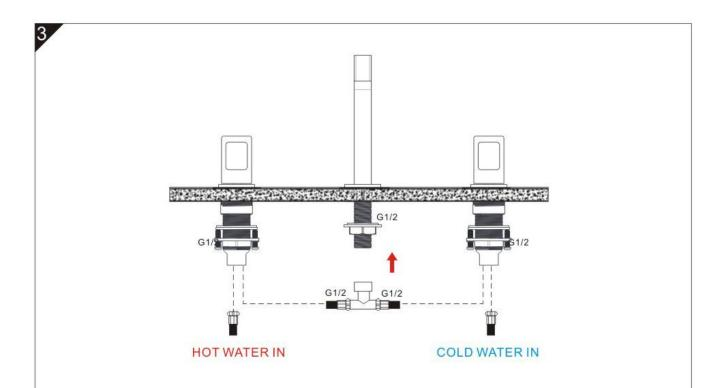
Connect one side of the Inlet Hoses to the Control Water Bodies, the other side to Tee, and tighten them. The red hose is for hot water and the blue hose is for cold water.
