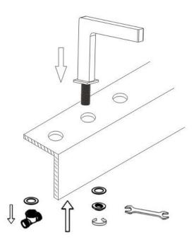
Connect Brass Part with Faucet Body and put the Brass Part through the basin hole. Install Faucet Body Gasket and Mounting Nut in sequence and tighten the nut with a wrench. Then put Tee Gasket into Tee and connect Tee to Brass Part.
