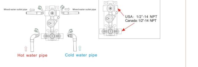
to the correct direction of installing the pre-buried main body. 2. Install the hot and cold water inlet pipes, Shower head and hand shower holder body jet pipes. Turn on the water source to test whether the left and right inlet pipes are tightly connected without leakage. After the test, adjust the flow switch to be on to test whether the mixed outlet pipe. The connection is tight and there is no leakage.
