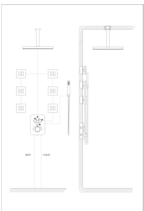
As shown in the figure, install the control valve, and fix the thermostatic control valwith the screws that originally removed the flap. After fixing the control valve, open the water pipe switch. Please pay attentio to check whether there is any leakage bet the control valve and the base. Control the valve and check whether the 6 rubber ring under the control valve are installed
