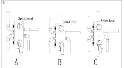
As shown in the figure, our company's embedded box has a built-in spirit level to correct the installation of the embedded box. It is best to move the mercury to the center of the spirit level. If it is not installed properly, it will affect the panel installation effect.
