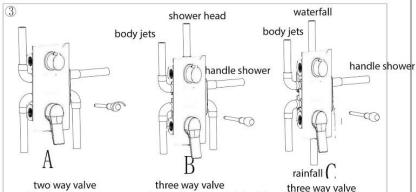
Open the water source to test whether the left and right inlet pipes are connected tightlyand without leakage. After the inlet pipe is tested, adjust the flow switch to be on to test whether the mixed water outlet pipes are tightly connected without leakage. At the same time, the water retention function is installed according to the embedded box. Built-in box with self-tapping screws in solid wall is fixed on the wall.
