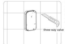
As shown in the figure, the external leakage embedded box is cut off, and the subsequent control valve installation can be performed after the wall is laid.
