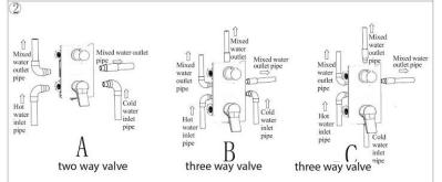
As shown in the figure, the inlet and outlet pipes are embedded. Pay attention to the correct direction of installing the embedded box. Be sure to mark the top  $\mathbb{TQP}$  of the baffle upward, and the vertical direction of the embedded box. The lower left interface is connected to the hot water pipe. The interface is connected to the cold water pipe, the upper left interface is connected to the top spray pipe, and the upper right interface is connected to the handheld pipe.
