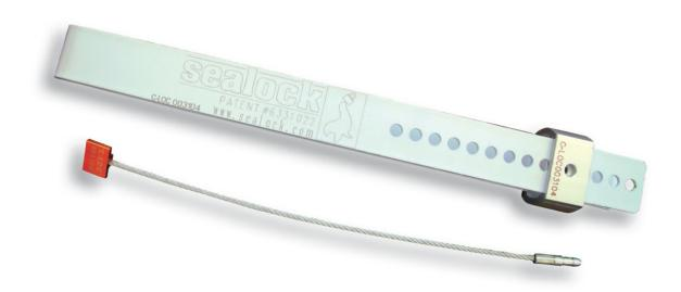
Made of 51mm wide steel that is 6mm thick, the Sealock Model SU2013 requires two cuts and two tools to remove. This need for both a power cutting tool such as an angle grinder and a cable cutter prevents break-ins by thieves who generally do not carry such sophisticated tools with them.
