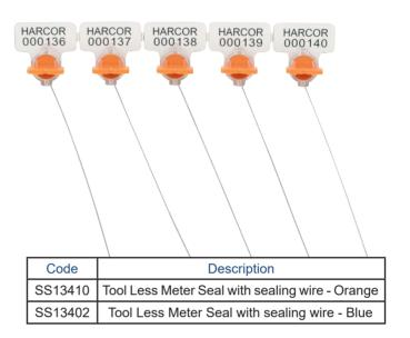
**Usage Instructions:** Start by feeding the sealing wire through the seal's free orifice. The tab on top of the seal is then twisted clockwise to secure the wire in place. Once secure the tab is to be removed by bending it in either direction.
