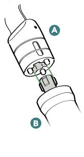
Twist the dial on the HUB to the OPEN position. Then, insert the HANDLE connector prong into the HUB.
