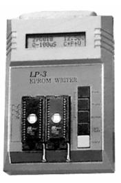
SUPPORTED DEVICES EPROM 27C64- 27C080 EEPROM 28C256-28C040 FLASH EPROM 29C256-29C040 29EE/LE512-29EE/LE020 28F256-28F020A 28SF/VF 040 29F010-29F040 29F001-29F040 39SF/VF512-39SF/VF040 49F512-49BF040
