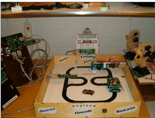
Formula Flowcode with an automatic timing system made with E-blocks and RFID cards.
