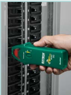
Adjustable sensitivity for pinpointing the correct breaker
