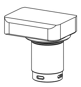
STEP 2 START MACHINE PUMP. INDICATOR WILL CHANGE FROM GREEN -> RED -> YELLOW. ONCE IT TURNS YELLOW, STOP PUMP AND ALLOW THE BACKFLUSH TO BEGIN. IT MAY TAKE 30 SECONDS OR SO TO COMPLETE. AFTER THE INDICATOR TURNS BACK TO GREEN, WAIT ANOTHER IO SECONDS AND MAKE SURE THE MACHINE PRESSURE IS AT O. USE CAUTION WHEN REMOVING SPRING CLEAN - YOU MAY WISH TO USE A RUBBER DISHWASHING GLOVE TO PREVENT HOT WATER FROM SPILLING ONTO HANDS.
