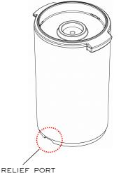
THE SPRING CLEAN™ WAS INVENTED AND DESIGNED TO IMPROVE THE BACKFLUSH PROCESS BY GENERATING SIGNIFICANTLY MORE WATER FLOW BACK THROUGH THE BREW LINES AND THE 3-WAY SOLENOID VALVE OF 58MM PORTAFILTER COMMERCIAL ESPRESSO MACHINES. BY USING MORE WATER, THE RESULT IS A CLEANER AND BETTER FUNCTIONING MACHINE. CAN ALSO BE USED BETWEEN SHOTS WHILE CHANGING BEAN TYPES TO PREVENT ANY LINE CONTAMINATION THAT MAY AFFECT FLAVOR.
