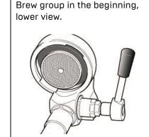
Use a flat screwdriver to pry out the shower screen and the group gasket.
