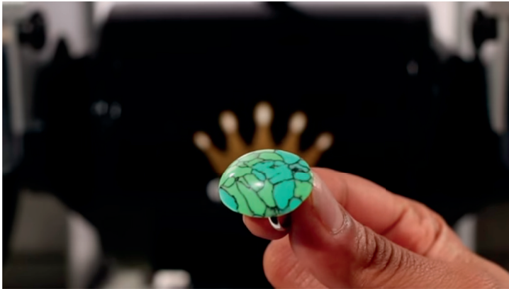
Polishing green turquoise on the CabKing cabbing machine
