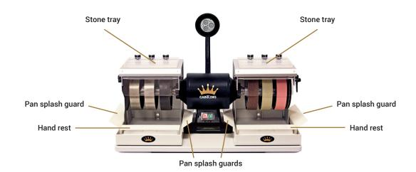
Refer to diagram above for assembly. Determine a suitable, well lit location to place your CabKing-6V3. The machine weighs about 60lbs. You need a sturdy table or stable surface that has 3 feet width by 2 feet depth of clear space.
